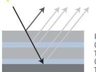
Protective glass Optical bonding Touch screen Optical bonding TFT display
